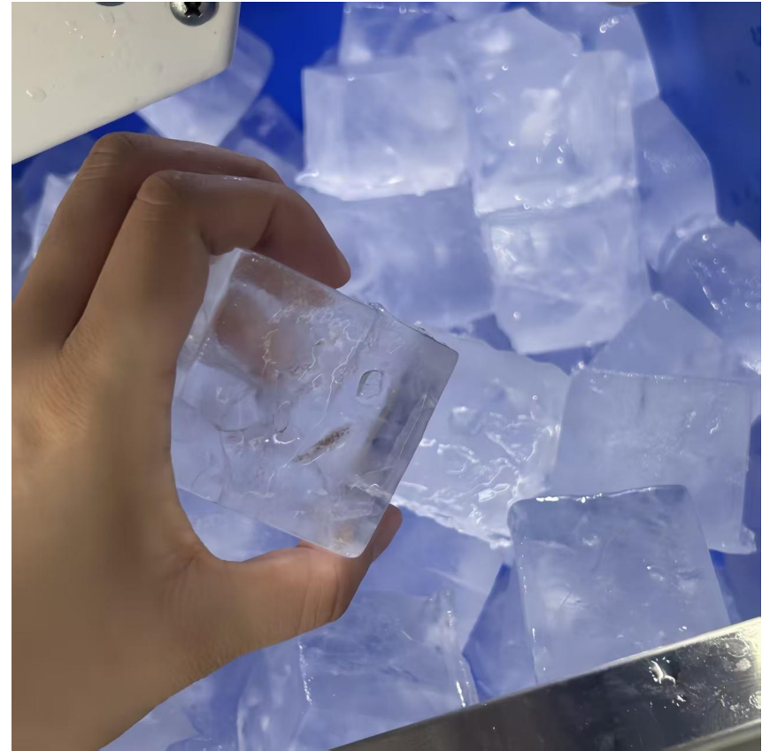
50mm x 50mm x 50mm clear cube ice formed in 20 minutes
